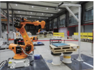
Recognition and Grasping of Condenser Tubes
