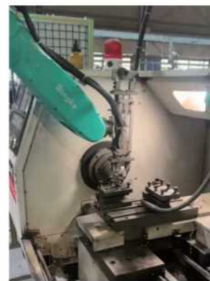
Linear machine tool loading & unloading
