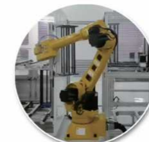
Photovoltaic basket handling
