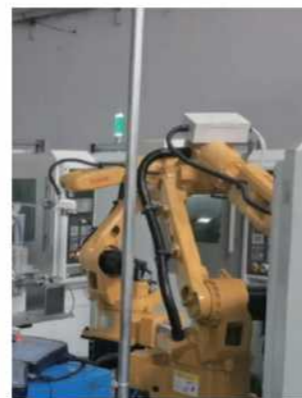
Island-type machine tool loading & unloading
